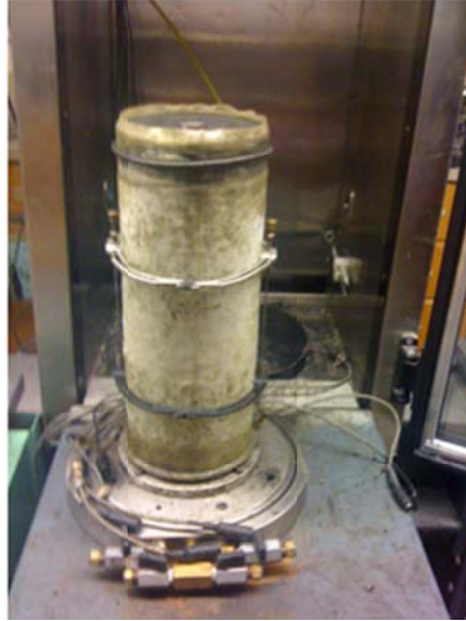
Figure 4 LVDTs used for measuring the permanent deformation
