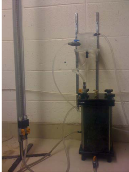
Figure 5 Constant-head Permeability Test Equipment
