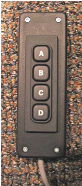
Figure 21. Remote Control Used for Initiating Wind Gusts
