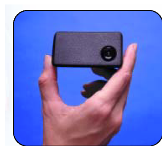
Figure 3. Lane departure camera windshield mount unit
