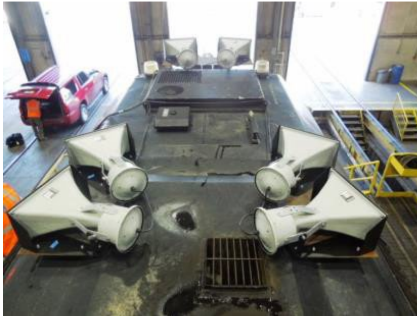
Figure 24. Top View of AWD System Six Speakers Installed on TTCI's DOTX4113 Locomotive
