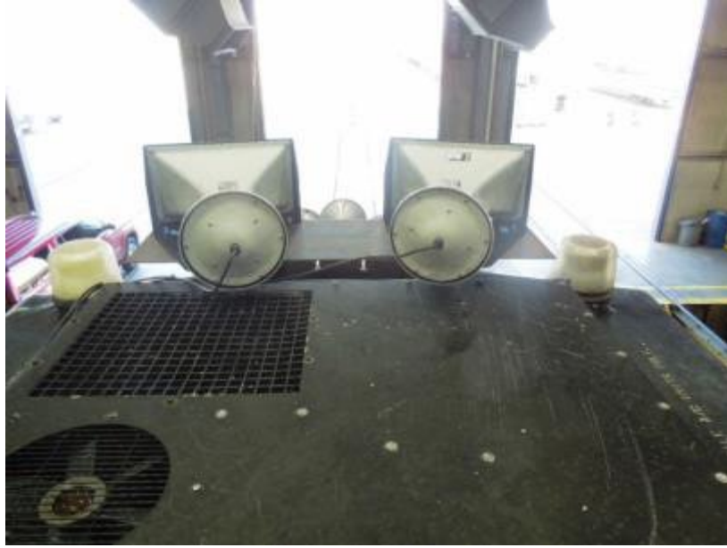
Figure 23. Two AWD Speakers Located at \pm 15 Degrees Above the K5LA Air-pressure Horn
