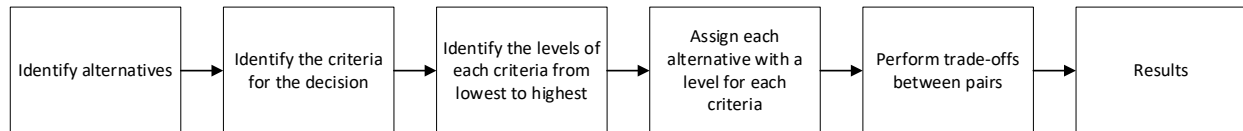
Figure 4.2: The Sequence of Steps in Performing the PAPRIKA Method in 1000minds Software
