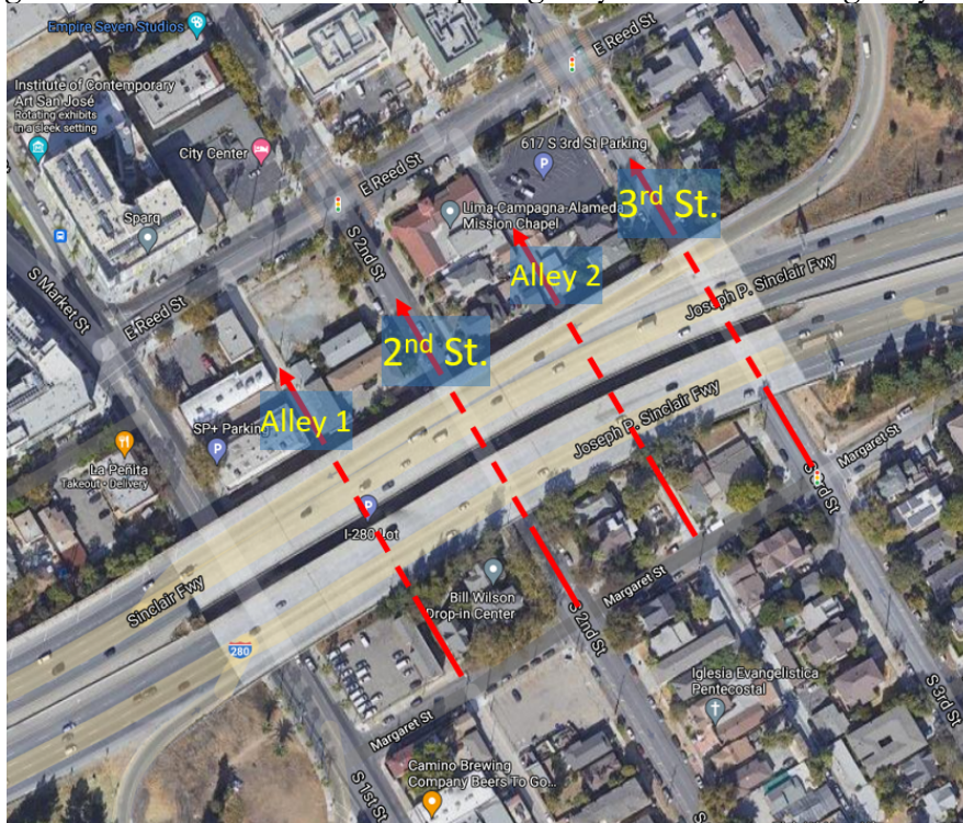
Figure 30. The four most feasible passageways underneath Highway 280.
