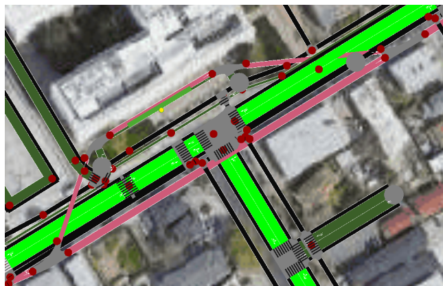
Figure A14. Setting edge points in SUMOPy.
