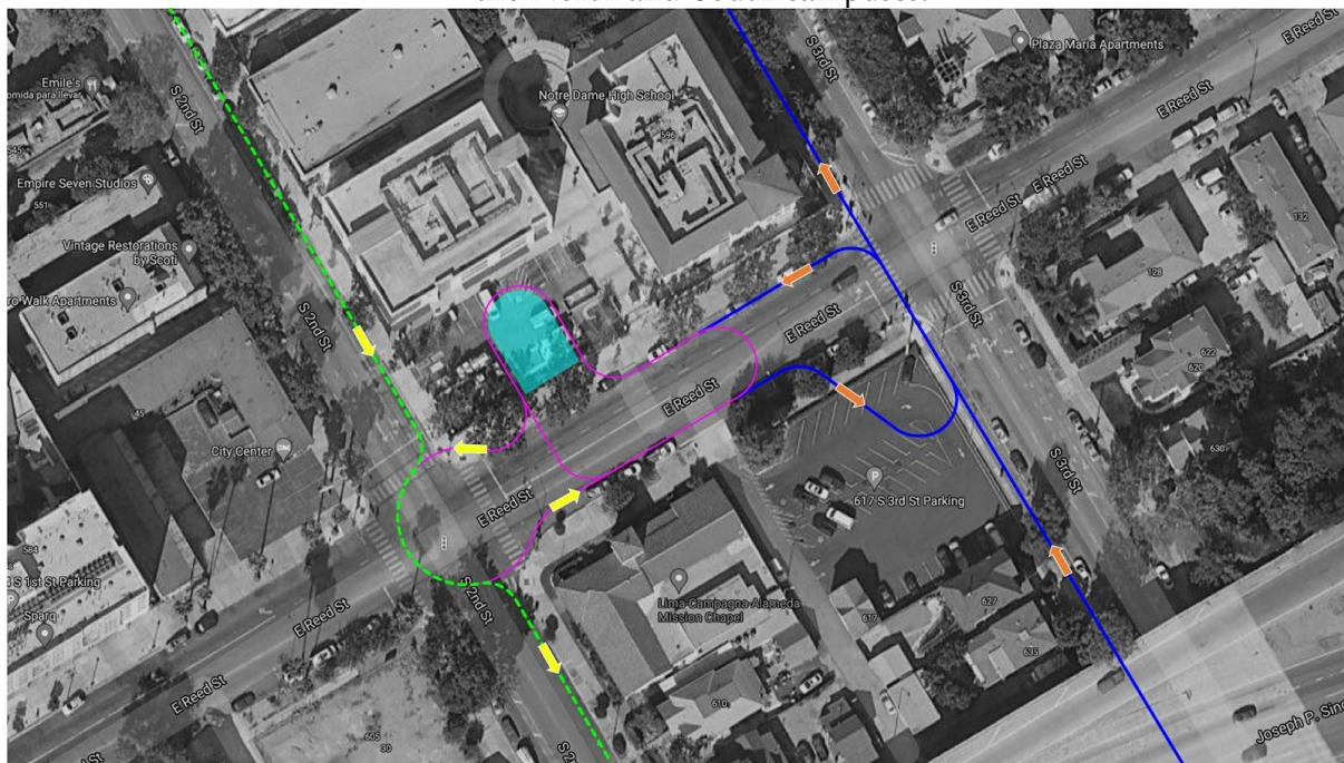
Figure 42. Placement of a single station servicing one-way guideways between the North and South campuses.
