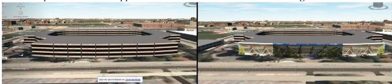
Figure C12. CEFCU Stadium in InfraWorks before (left) and after (right) photos have been applied to the side of the stadium model facing the viewer.
