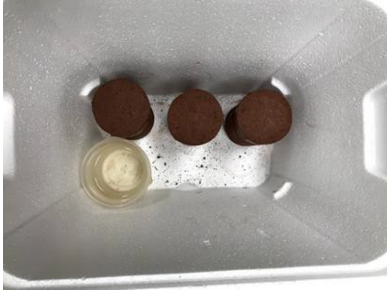
Figure 6: Curing of the soil-cement specimens
