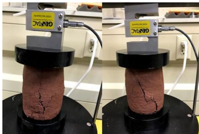
Figure 18: Failure mechanism of the control group (no cement) using 10% MC
