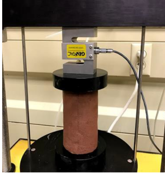
Figure 7: Set-up for a uniaxial unconfined compressive strength test.
