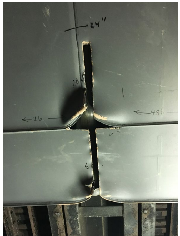
Figure 15. Post-test Photograph of DMU Fuel Tank; Bottom of Tank
