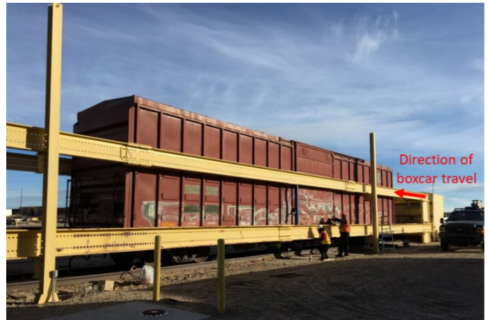
Figure 9. Box Car Positioned in Squeeze Frame Prior to Test
