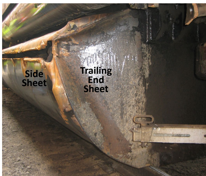
Figure 4. Damage to Trailing Locomotive Fuel Tank
