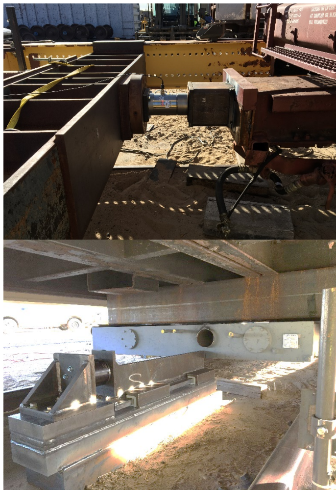
Figure 12. Load Cells Measuring the Load Applied (top) and Load Reacted (bottom)
