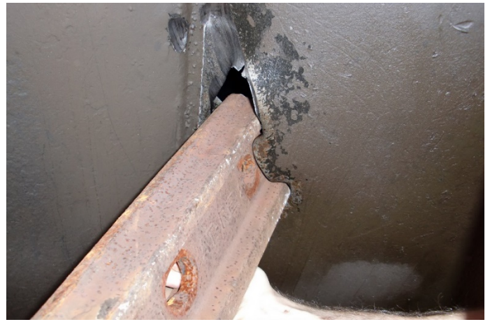
Figure 12. Identified Impact Object, an Exemplar Joint Bar Section and Joint Bar Inserted into the Fuel Tank Puncture Matches the Exact Contour
