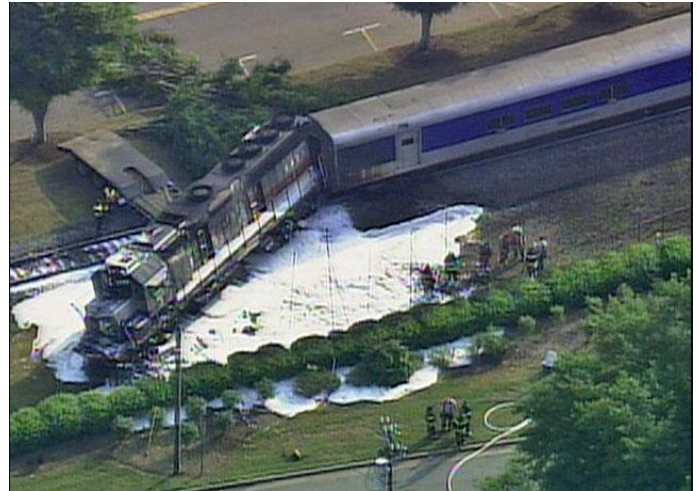
Figure 8. Photo Showing Locomotive Derailed with Tractor-trailer Lowboy Underneath. (Photo Source: WRAL.com)
