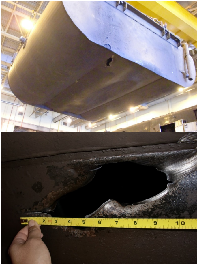
Figure 10. Puncture on Bottom Sheet (Concord, MA)
