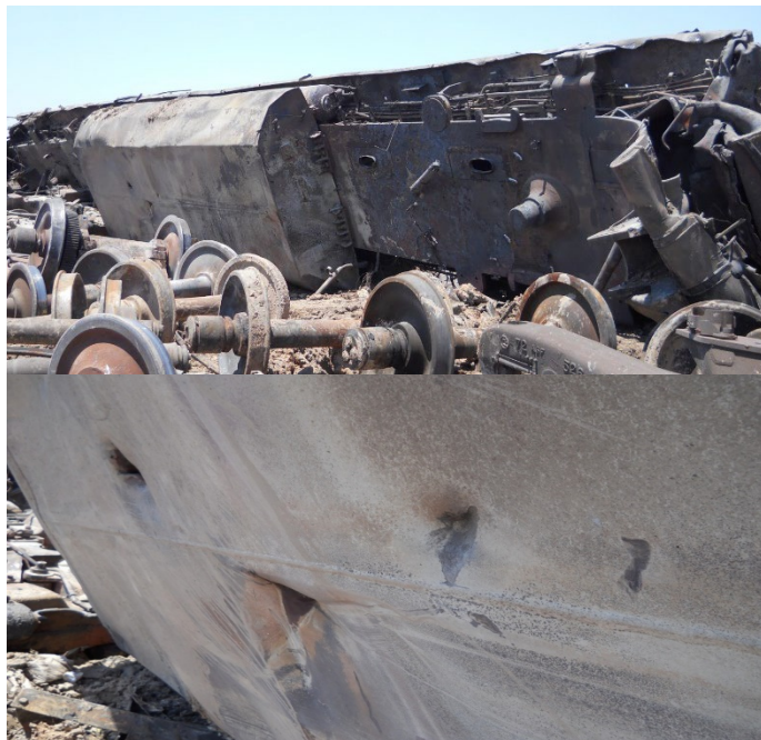
Figure 17. Post-collision Photos of Lead Locomotive, UP8542 Fuel Tank
