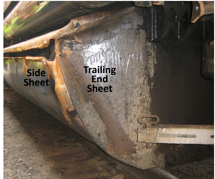
Figure 15. Damage to Trailing Locomotive Fuel Tank
