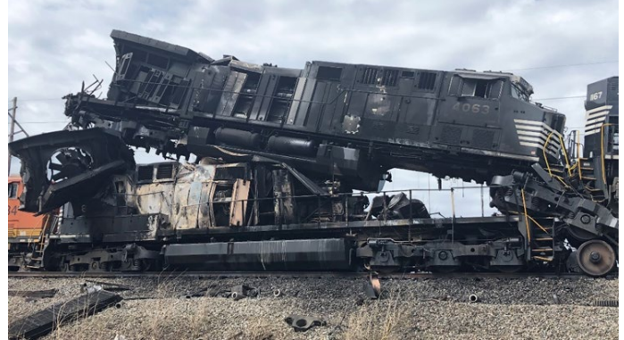
Figure 22. Post-accident Photo Showing Override of Second Locomotive on Leading Locomotive of Freight Train 175T817 (on Left) and Lead Locomotive of Freight Train M74T817 (on Right)
