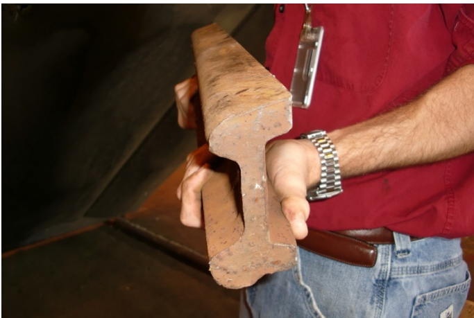
Figure 11. Identified Impact Object, an Exemplar Joint Bar Section
