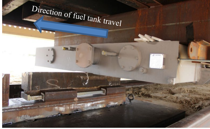
Figure 9. Fuel Tank and Indenter Setup for Second Raking Test
