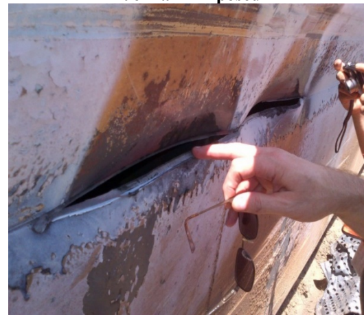
Figure 6. Close-up of UP4855 Fuel Tank Puncture
