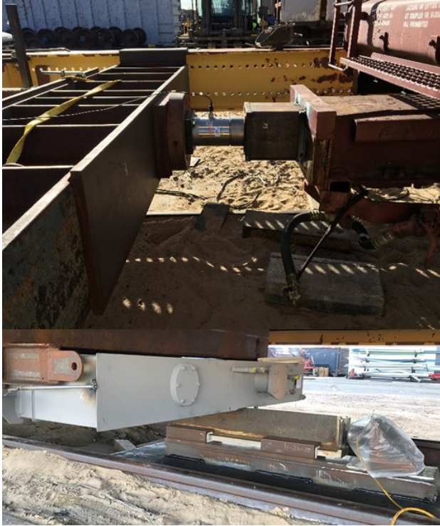
Figure 11. Load Cells Measuring the Applied Load (Top) and Reacted Load (Bottom)
