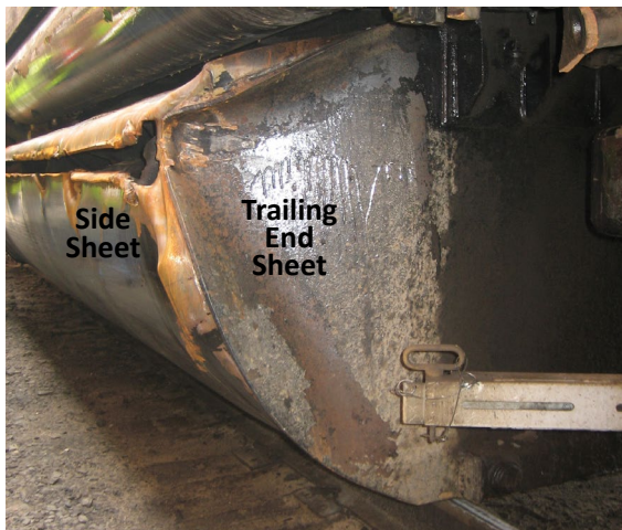
Figure 4. Damage to Trailing Locomotive Fuel Tank
