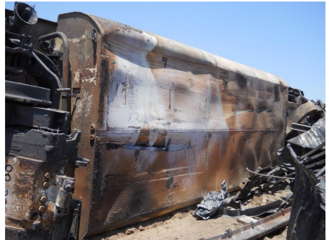
Figure 5. UP4855 Locomotive, Rolled Over with Bottom of Fuel Tank Exposed
