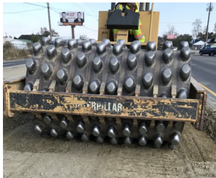
Figure 12. Pad foot roller for compaction
