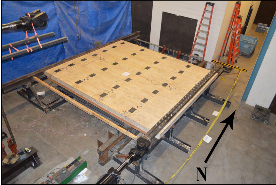
Figure 2.3 CLT Diaphragm Test Setup (View from a Top Angle)
