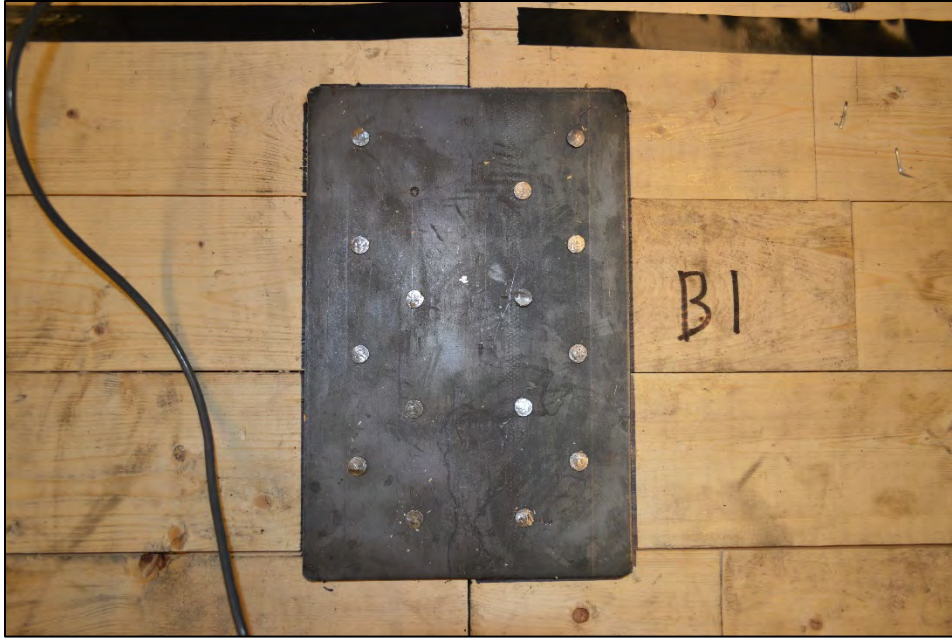
Figure 4.5 Connector B1 before the Test (Top View)
