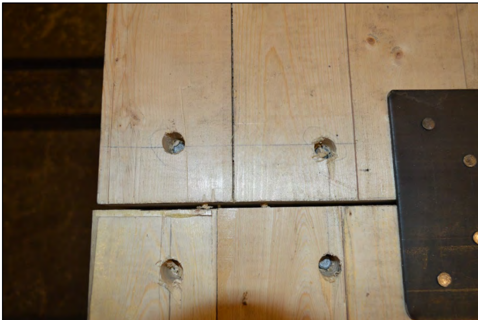
Figure 2.4 SDS Screws into CLT
