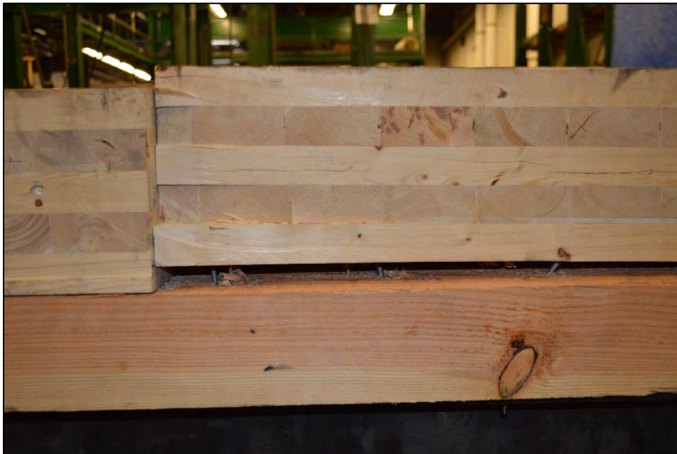
Figure 4.8 SDS Screw Shear Failure
