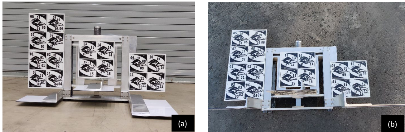
Figure 4-11: Placing the gage block (2''): (a) Y-direction, (b) Z-direction
