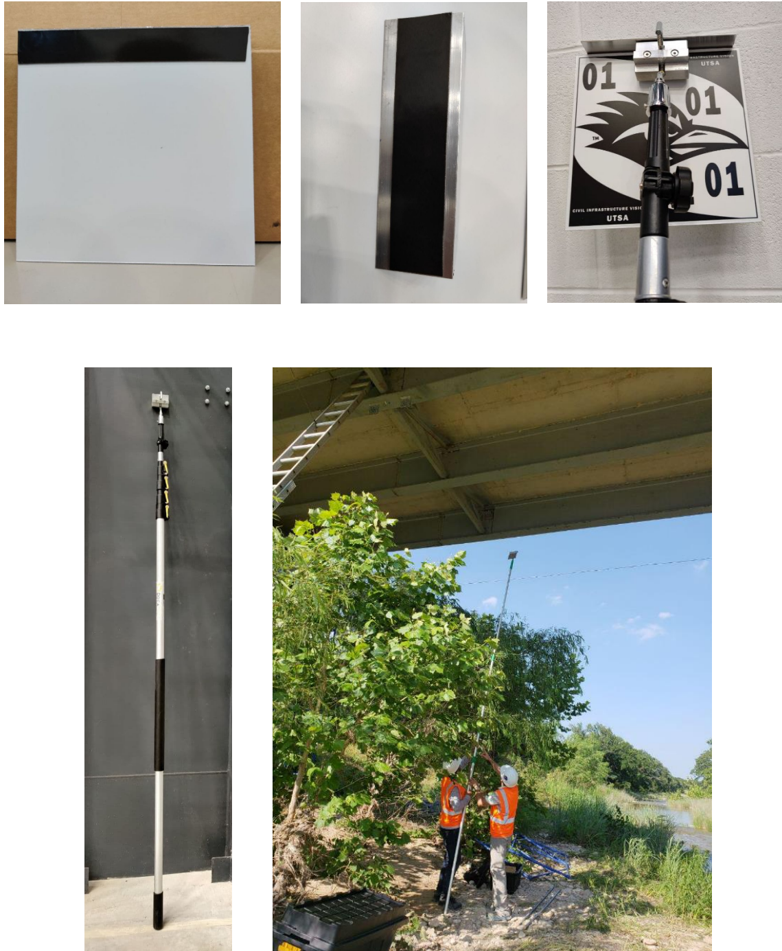
Figure 3-5: Double-sided tape on target and extension rod
