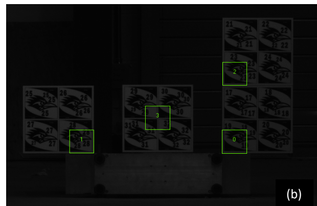
Figure 4-6: Reference axis target (Target 0, 1 and 2) and Center Target (Target 3): (a) Y-direction, (b) Z-direction
