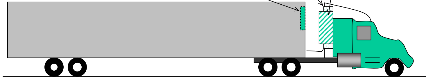
Layout of Adsorption Refrigeration System and Sorption Compressor on Tractor
