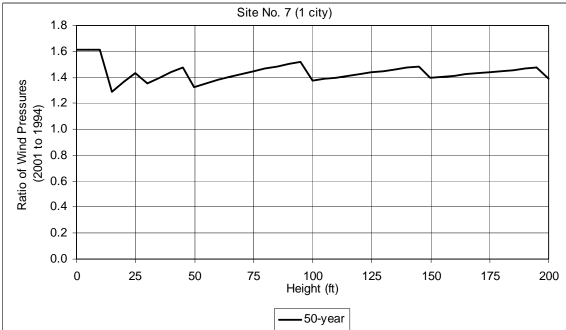
Figure 3-19. Site no. 7: ratio of wind pressures (2001 to 1994 specifications)
