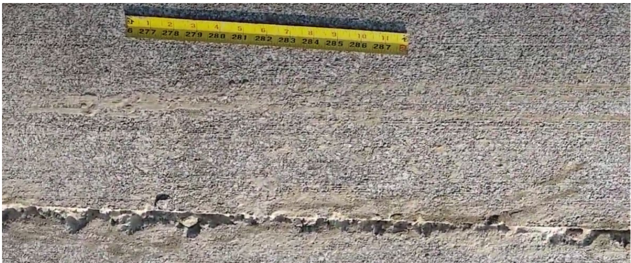
C. HVFAC mix: saw cut after 6 hours 20 minutes
