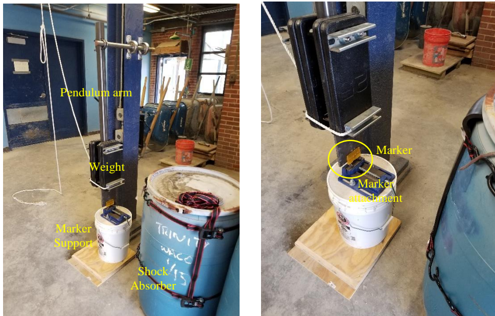
Figure 7-6 Laboratory pendulum impact testing setup for flexible memory markers
