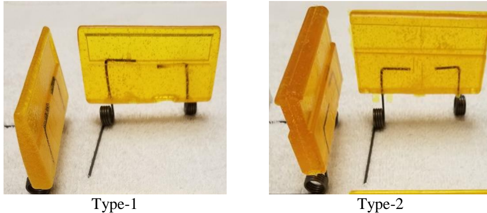
Figure 7-4 Examples of fabricated tapered and non-tapered markers with 90° deflection springs
