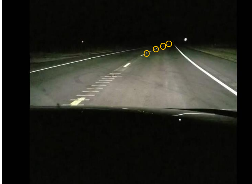
Figure 6-14 Qualitative visibility of RPMs in Location 1 (US 380, Wichita Falls District), illuminated markers circled
