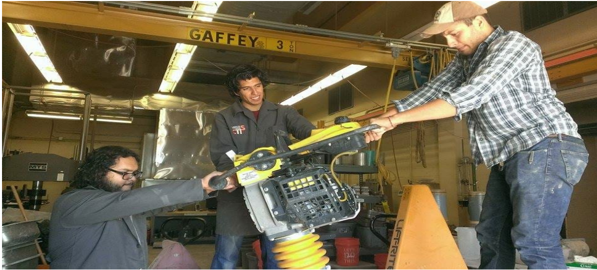
Figure 4-2 Sample Preparation Using Vibratory Compactor
