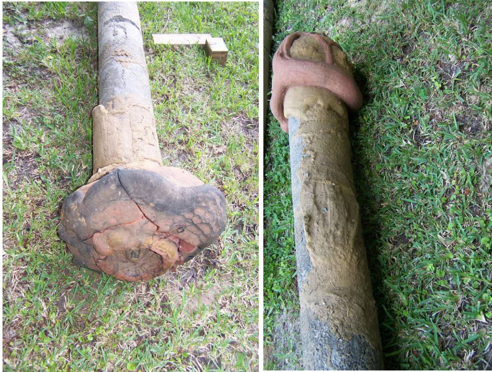
Figure 7-10 Excavated post-grouted shafts (Group test 2).
