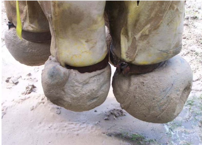
Figure 4-67 View of tip grout bulbs.
