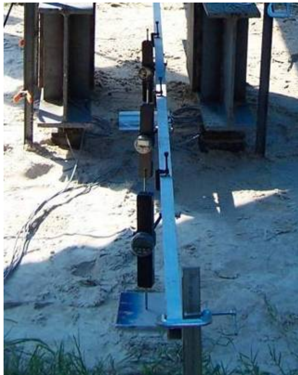
Figure 4-27 Digital dial gages for soil deformation monitoring.
