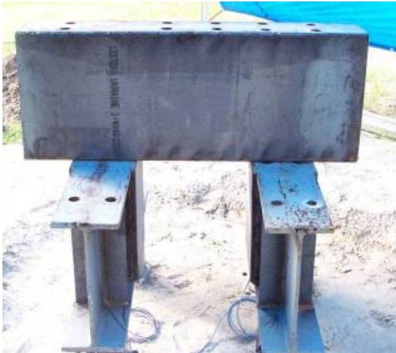
Figure 3-9 Grout test frame.
