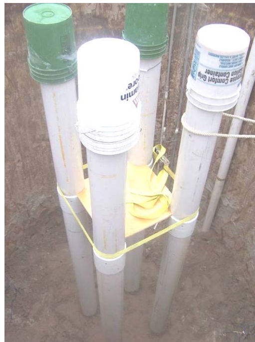
Figure 5-36 PVC casing positioned in the test chamber.
