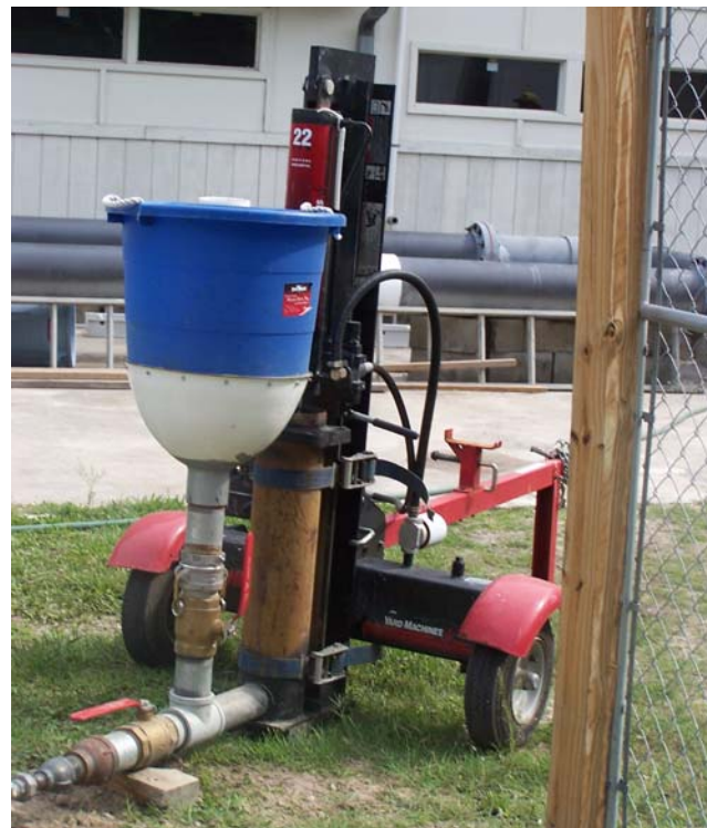
Figure 4-21 Grout pump with holding tank.
