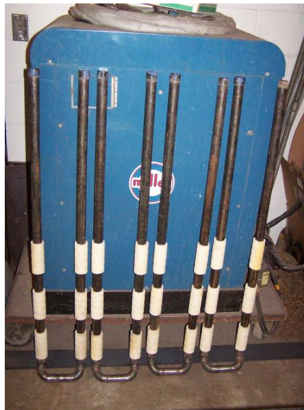
Figure 4-57 Side grout delivery system.
