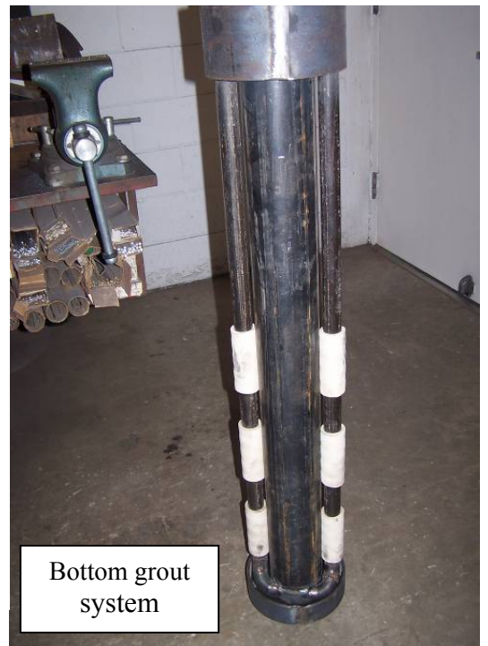
Figure 4-58 Pile with grout delivery systems.
