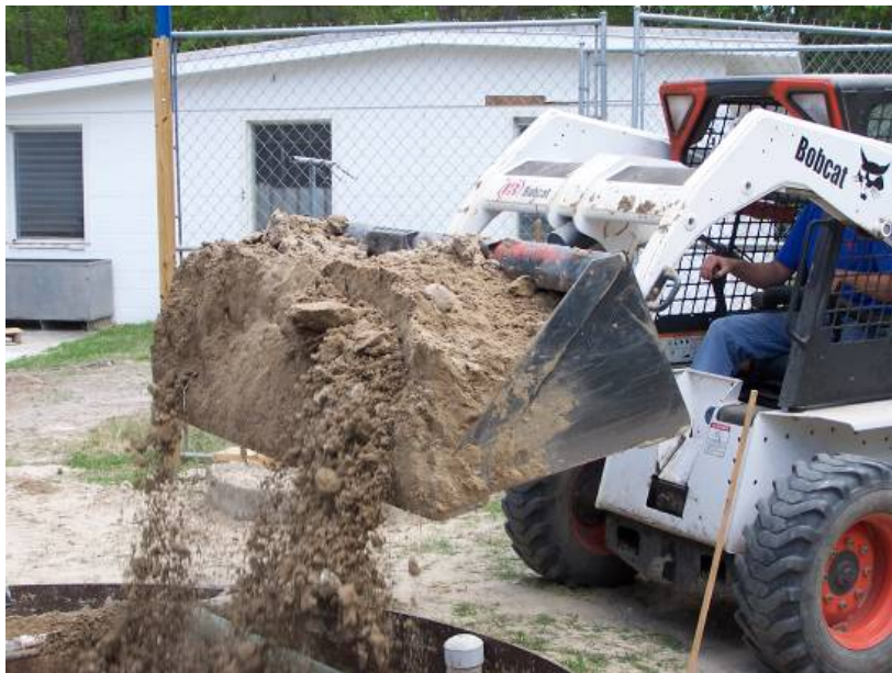
Figure 4-11 Filling test chamber with loose silty sand.
