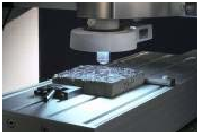
Figure 4. Polished Contrast Enhanced Concrete Plane Section under the Objective [14].
