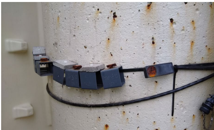
Figure B 7 - Specimens and probe under shields after one year of exposure
