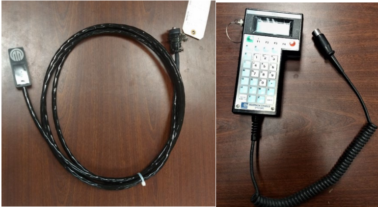
Figure B 4 - Corrosion probe and reader
