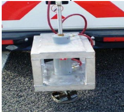
Figure C.8: Texas Field Torque Device (After Freeman et al.2010)
