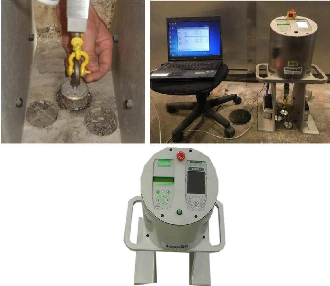
Figure C.5: Com-Ten Pull-off tester (After Mealiff et al. 2017).
