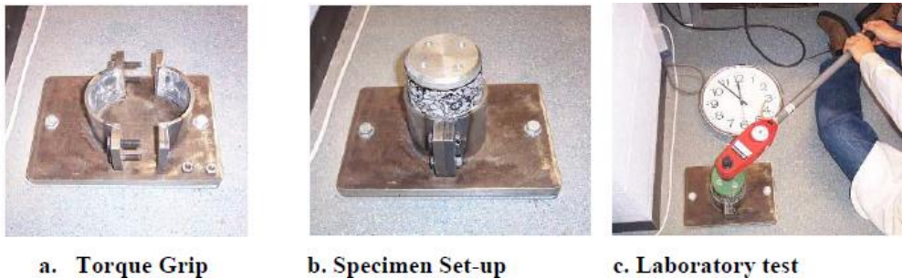
a. Torque Grip b. Specimen Set-up c. Laboratory test Figure C.7: Laboratory torque bond test. (a) Torque Grip, (b) Specimen Set-up, and (c) Laboratory Test
