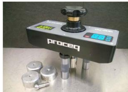
Figure 2. Proceq Dy-206 Pull-off Testing Device
