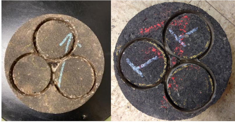
Figure C.3 Field core samples prepared for interlayer bond strength testing
