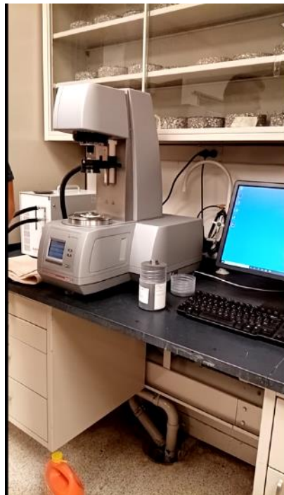
Figure A.13: Anton-Paar MCR 302 Dynamic Shear Rheometer (DSR) equipment used for measuring rheology of asphalt binder
