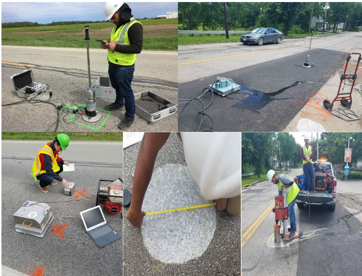
Figure A.3 Photographs taken during measuring the structural capacity and surface texture for both projects.
