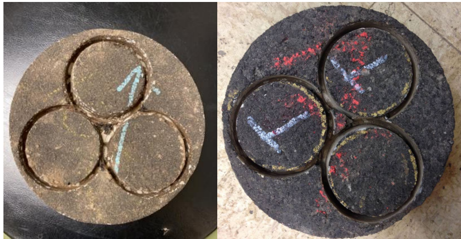
Figure A.7 Field core samples prepared for testing in the lab.
