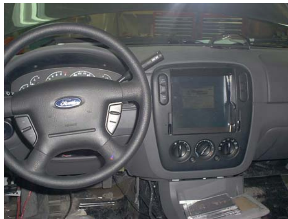
Figure 8 View of the touch screen, which replaced the radio in Summit.
