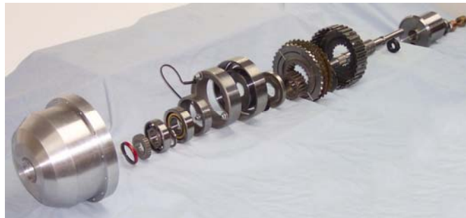
Figure 5: Four-wheel drive/all-wheel drive clutch assembly.
