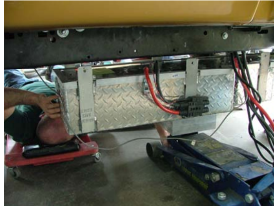
Figure 17: Capacitor pack installation.
