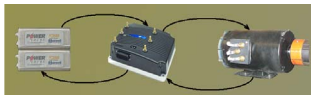
Figure 7: Motor controller and induction machine.
