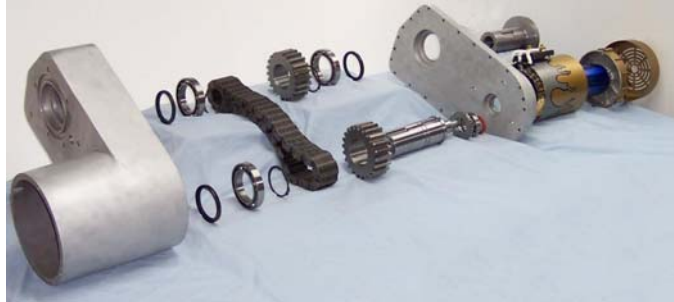
Figure 4: Housing, chain assembly and induction machine.
