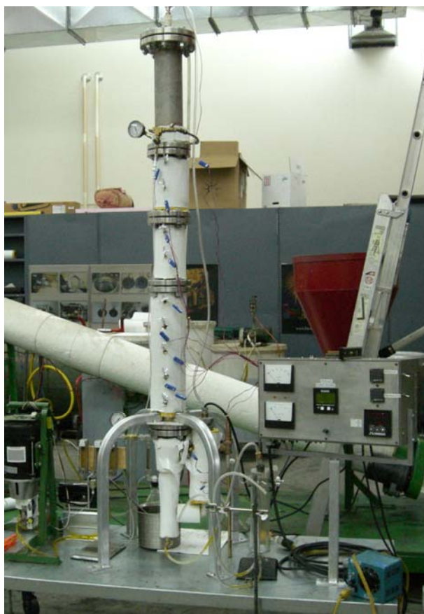
Figure 4. Bench-scale continuous-flow RD reactor unit for biodiesel production.
