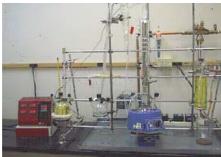
Figure 1. Experimental setup of the laboratory-scale continuous-flow RD reactor system.
