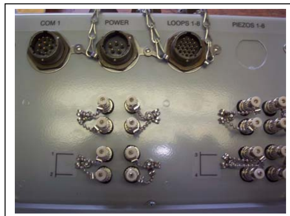
Figure 5: Side View of TCC-540 Showing Interface Connections
