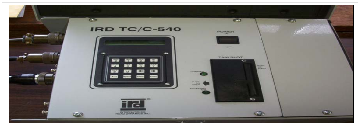
Figure 6: Front View of TCC-540 Showing Keypad, Power Switch, and Connections
