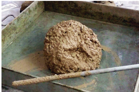
Concrete slump made of an alternative cementitious material (calcium sulfoaluminate). © College of Engineering, Georgia Institute of Technology.
