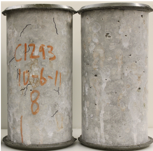
Two concrete samples using equivalently reactive aggregate. Left, ASR-damaged concrete with cracks marked; right, crack-resistant HyFRC for concrete strength and stiffness retention. © 2013 Claudia Ostertag.
