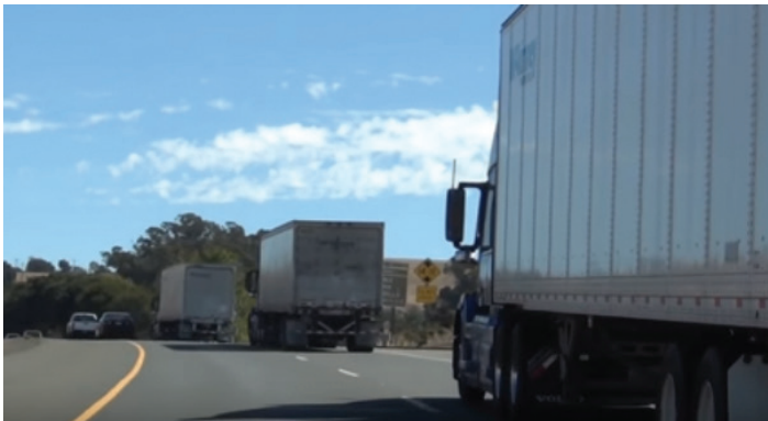
Three Class 8 trucks equipped with CACC during field test. © University of California, Berkeley.
