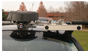
Camera and LIDAR equipment mounted on the roof of the test vehicle. Source: FHWA.
