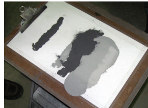
Fly ash with different carbon content levels. Source: FHWA.
