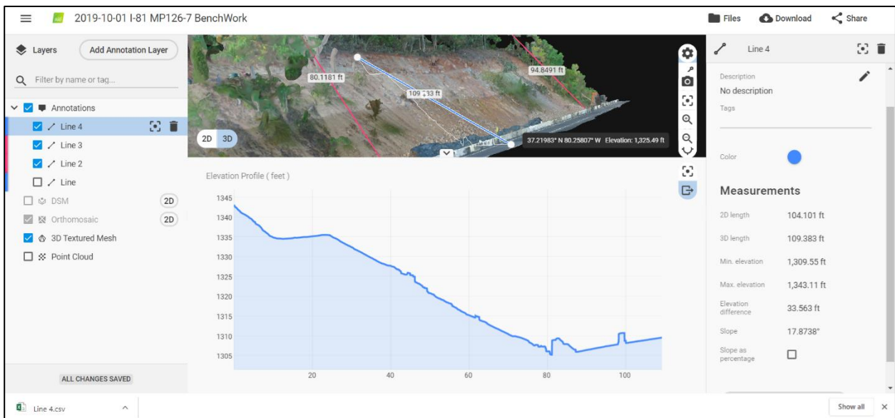
Figure 32. Site #6, Ironto, I-81 Milepost 126.7 Southbound; UAS demo project for GeoStabilization International. Measurements and profile section made on the dense point cloud generated in Pix4D Cloud . Note how the UAS 3D model picked up the Jersey barrier on the right side of the profile, the bundled rockfall mesh in the ditch, and some rock slabs resting on the slope face.
