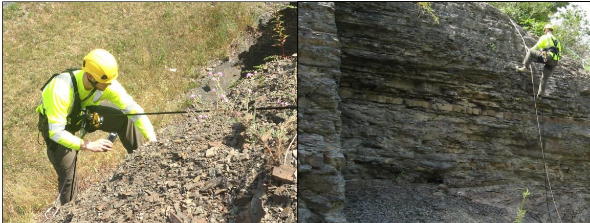
Figure 11. Graduate student Robert Huber using rope access to safely collect geologic structure data at the Deerfield site in the traditional manner. This method is less efficient than newer UAS techniques and can place personnel in hazardous situations.
