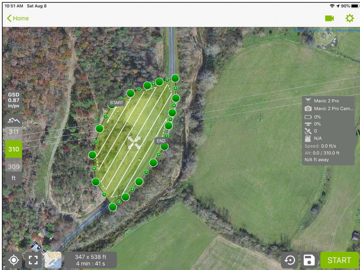
Figure 16. Site #2, Deerfield. Dots outline the imaged portion of the rock slope face. White lines represent the flight path of the aircraft as it flew directly over rock slope. The UAV camera was looking vertically downward for standard photogrammetric mapping. The flight control software was Pix4D Capture.
