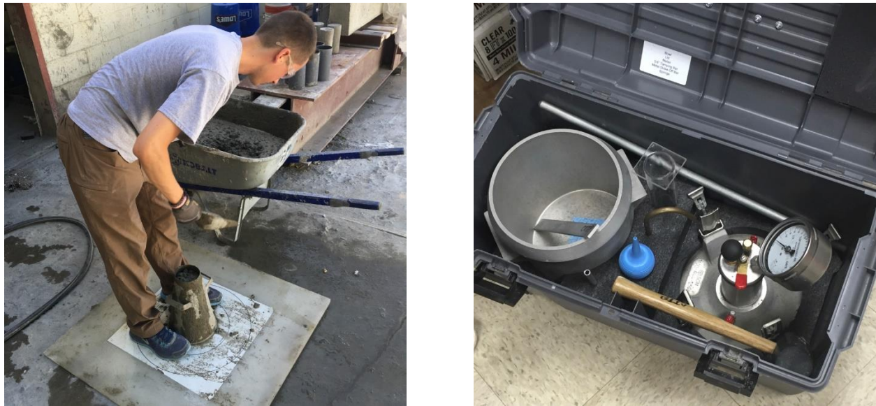
Figure 3.4 – Sump, Unit Weight, and Air Content Measurements
