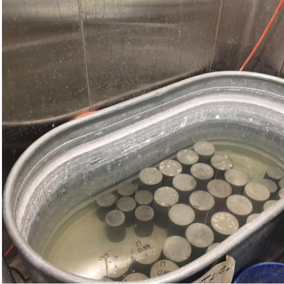
Figure 3.5 – Compressive Cylinder and Unrestrained Drying Shrinkage Prism Storage
