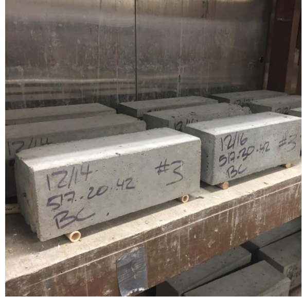
Figure 3.5 – Compressive Cylinder and Unrestrained Drying Shrinkage Prism Storage
