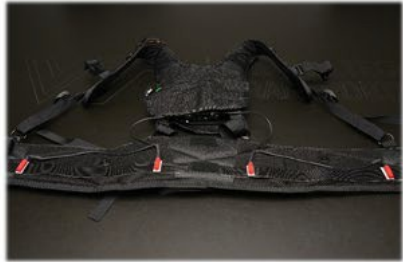
Smart Vest tactors attached to the belt using a Velcro strip allowing adjustments, if needed
