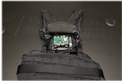
Smart Vest electronics are protected with a waterproof fabric and neoprene which are secured using snap on buttons
