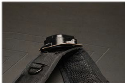
Smart Vest GPS antenna with ground plane attached to harness using snap on button
