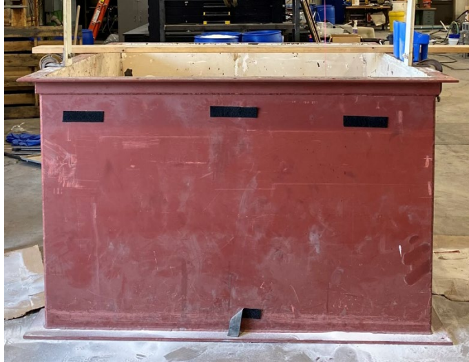
Figure 3.9. Test box used for laboratory study.
