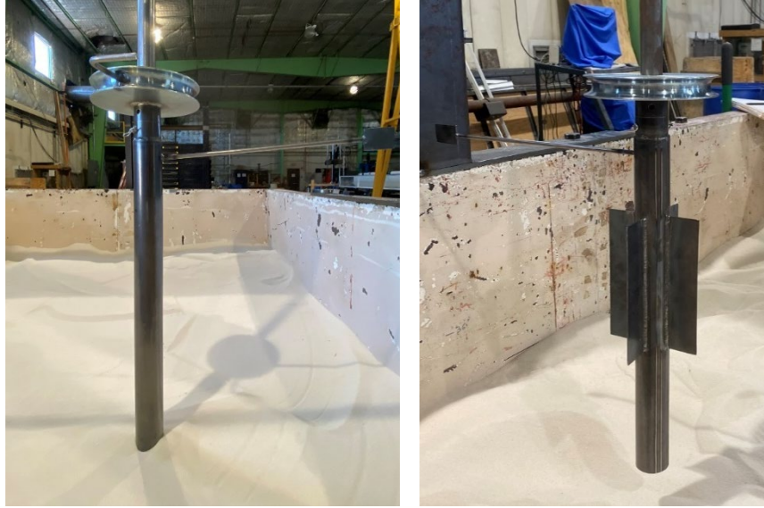
Figure 3.12. Piles tested in the laboratory: (a) unfinned pile; (b) fin pile.
