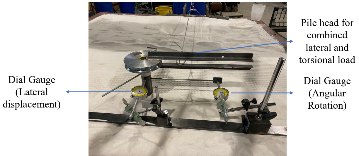
Figure 3.18. Combined torsional and lateral load test setup loaded at an arm length of 15 cm.
