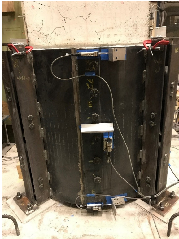
Figure 4.8: Shell splice instrumentation
