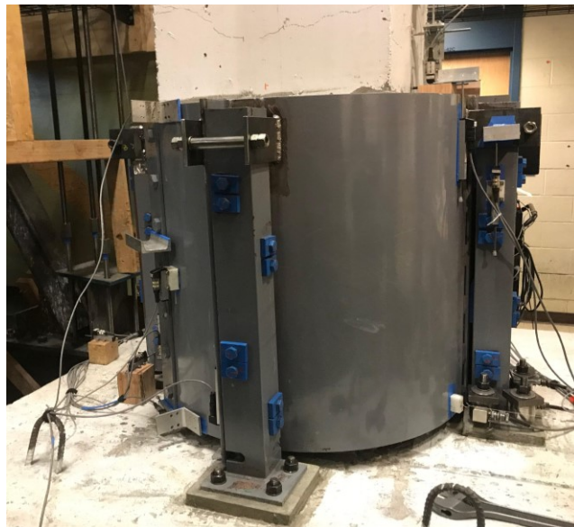
Figure 5.8: Test 3 modification - hold-down roller
