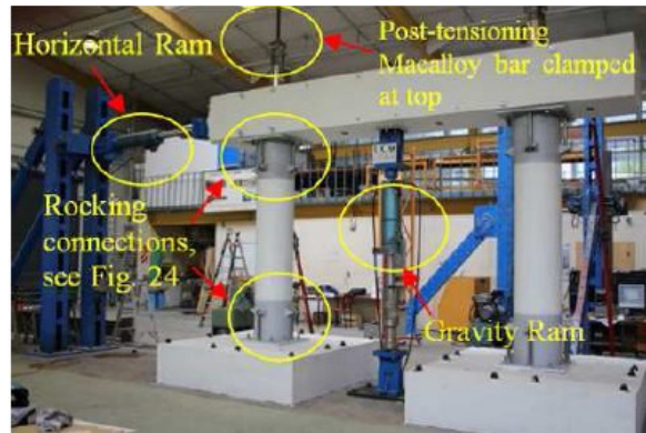
Figure 2.7: Test configuration (Mashal et al. 2014)
