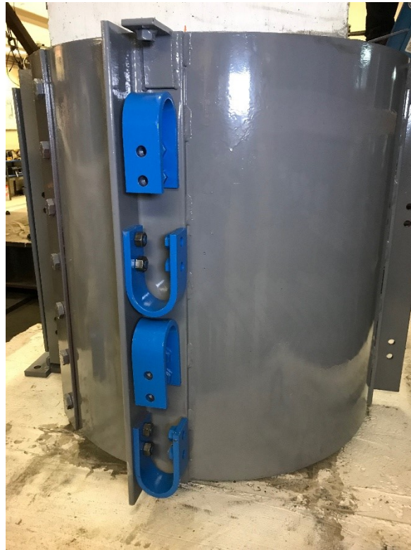
Figure 4.4: UFPs inside hold-down
