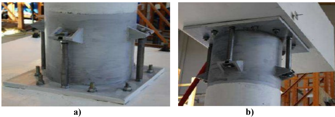
Figure 2.8: (a) Lower rocking interface, (b) Upper rocking face (Mashal et al. 2014)
