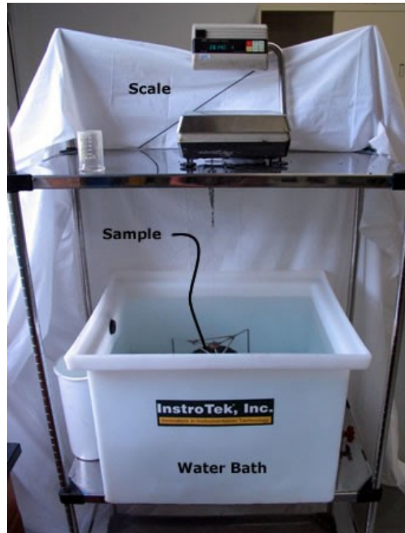
Figure 2.23. Saturated surface dry (SSD) test (Source: www.pavementinteractive.org )
