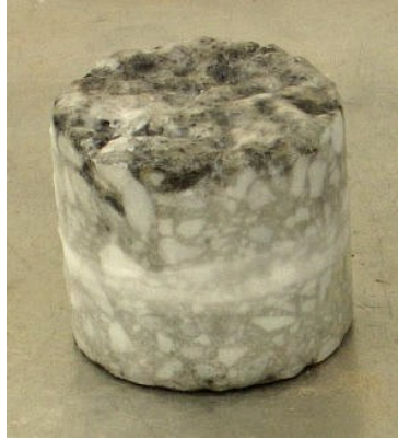
Figure 2.26. Paraffin-covered HMA specimen (Source: www.pavementinteractive.org )
