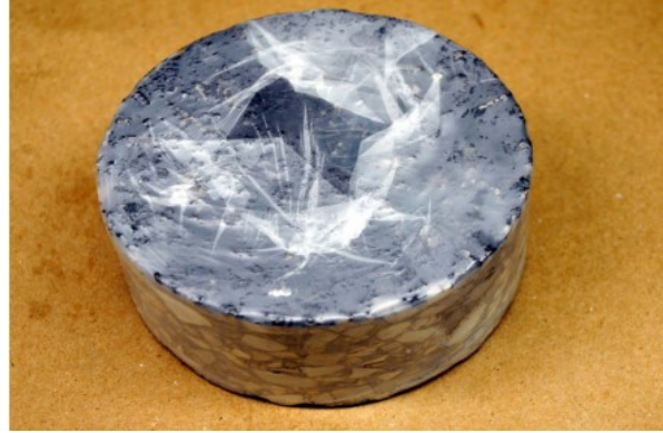
Figure 2.27. HMA specimen covered with Parafilm (Schroer 2012)
