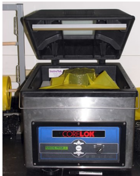
Figure 2.29. CoreLok vacuum chamber (Source: www.pavementinteractive.org )
