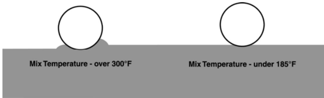
Figure 2.14. High temperature increases the possibility of achieving higher density (Decker 2006) Temperature conversion: [C=(F-32)/1.8]
