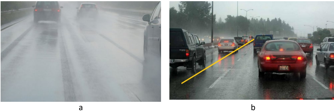
Figure 5. Rain marks and stationary vehicles identified as lane boundaries
