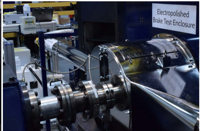
Fig 3: Inlet duct (left) and return duct (right) with air moving in the right-to-left direction
