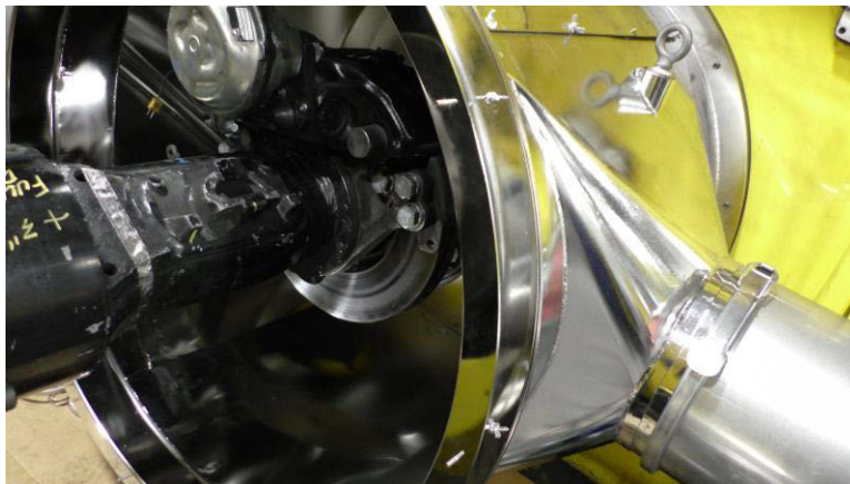
Fig 5: Air disc brake assembly mounted inside the enclosure
