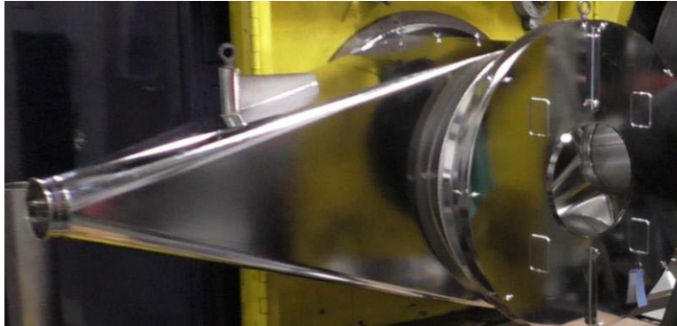
Fig 2: Aerodynamic brake enclosure exit (using a gentle transition angle to reduce transport losses)
