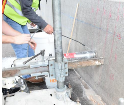
Figure 5.5: Set-up for core extraction
