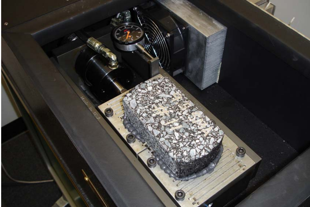
Figure 7 – Picture of the Overlay Tester (Chamber Door Open)
