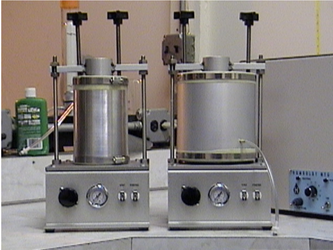
Figure 3 – Falling Head Permeability (4 and 6 Inch Diameter) for Asphalt Samples
