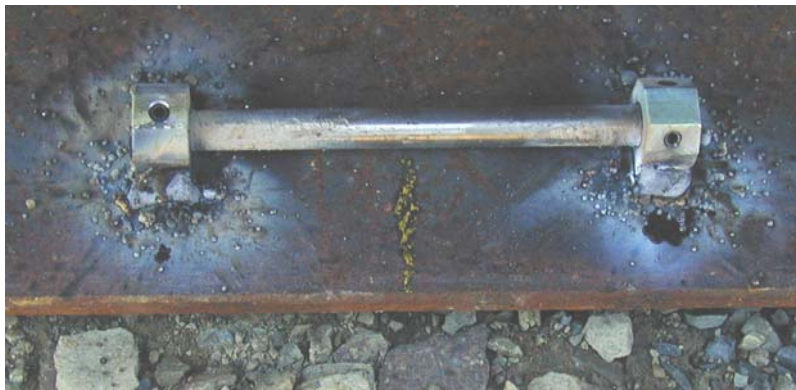
Figure 2.20: Photograph of Strain Gage on H-Pile After Welding
