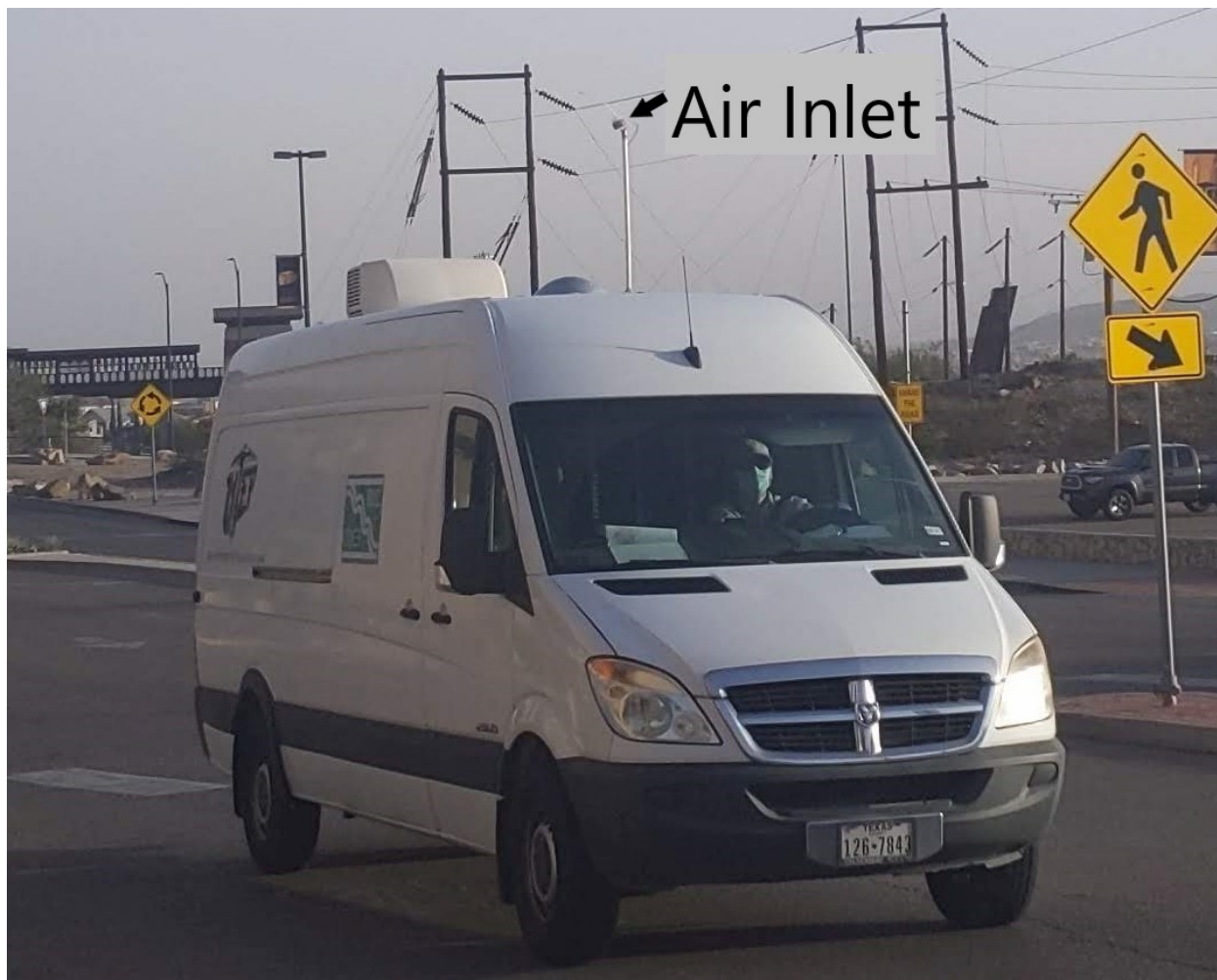
Figure 1 Air Quality Mobile Station
