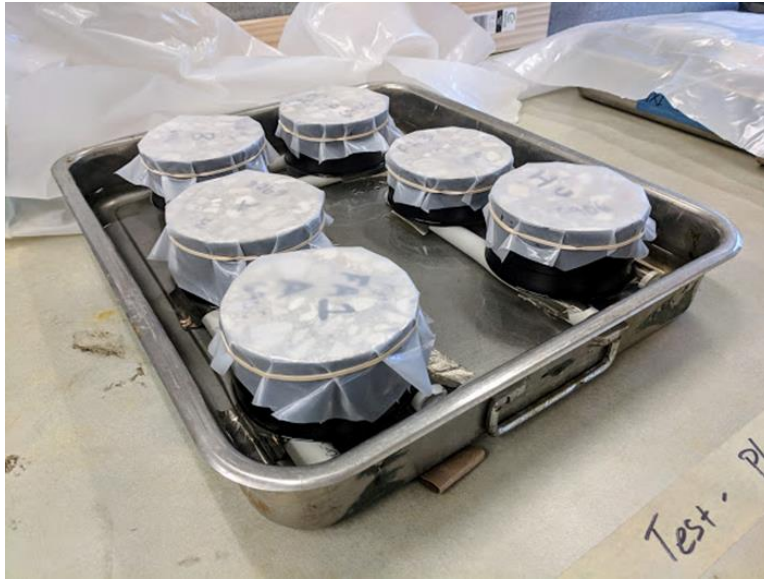
Figure 4.14 ASTM C1585 absorption samples
