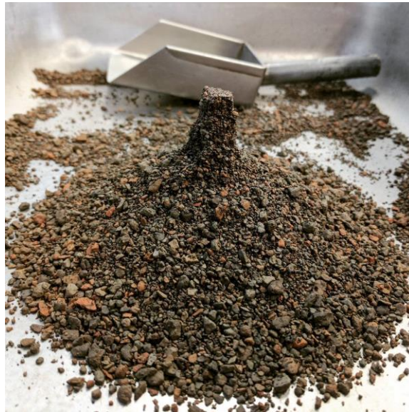
Figure 2.14 ASTM C128 cone test performed on LWFA
