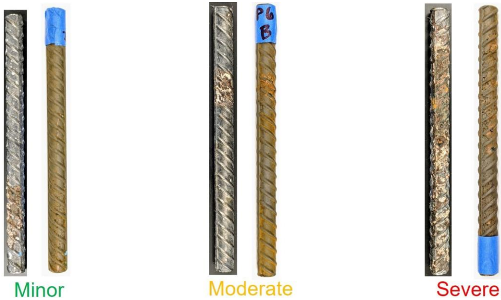
Figure 3.18 Rebar visual rating example—after removal from corrosion beam (left sample) and after cleaning procedure (right sample)
