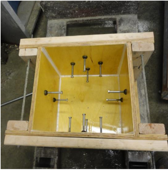
Figure 2.8 ASR exposure block form in new condition (left) and locations of exposure sites in Texas (right)
