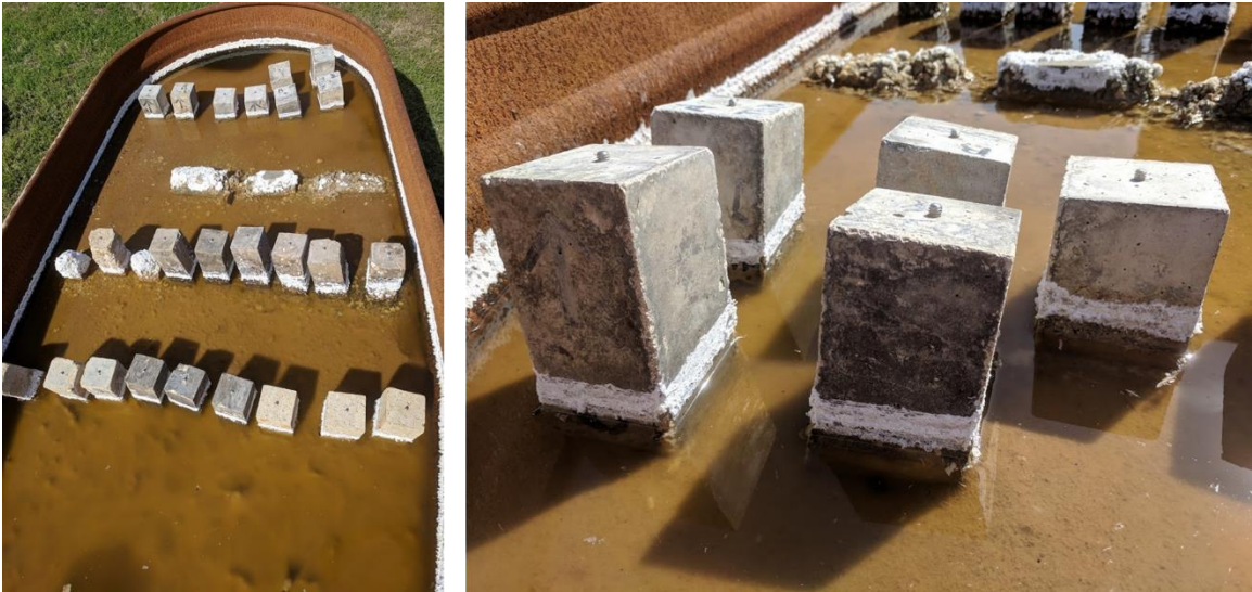
Figure 4.3 Outdoors trough at Central Texas Exposure Site. Contains submerged and standing prisms exposed to soil doped with sodium sulfate.
