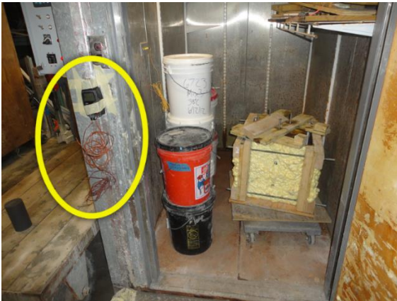
Figure 2.7 Preheating process in environmental chamber with thermocouple system highlighted (left) and mixing of Cooked block (right)
