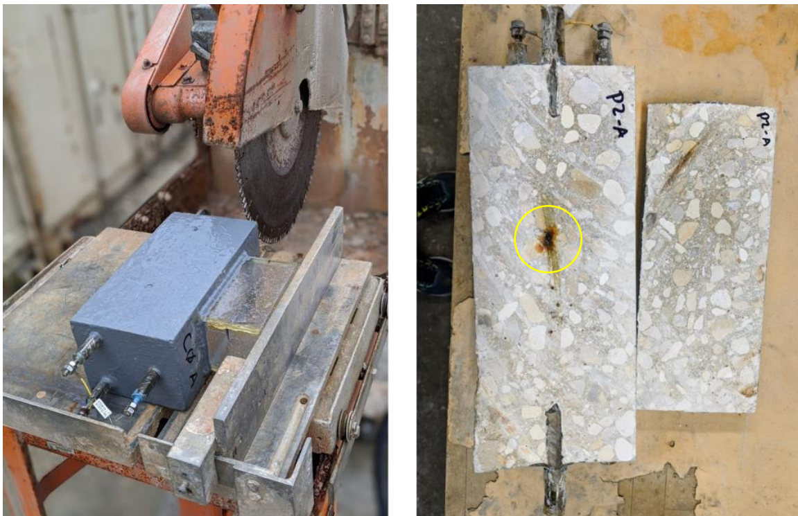
Figure 3.14 Saw-cutting corrosion beams (left), and rust staining visible after saw-cutting (right)
