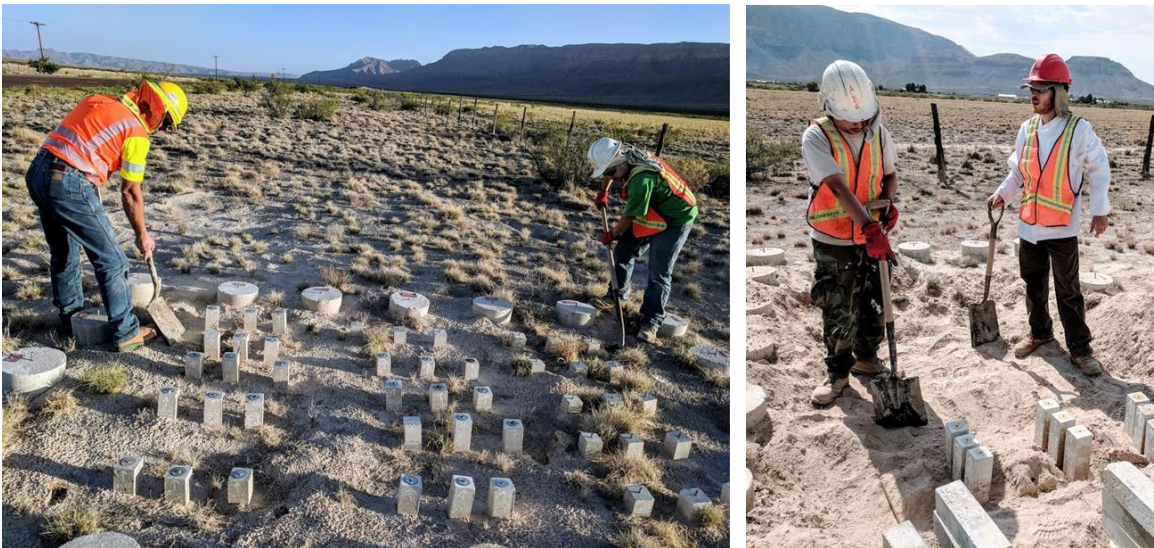
Figure 4.4 Site 1 in Van Horn (sodium sulfate environment)
