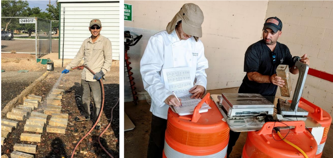
Figure 4.7 Samples being rinsed (left) and measured (right)
