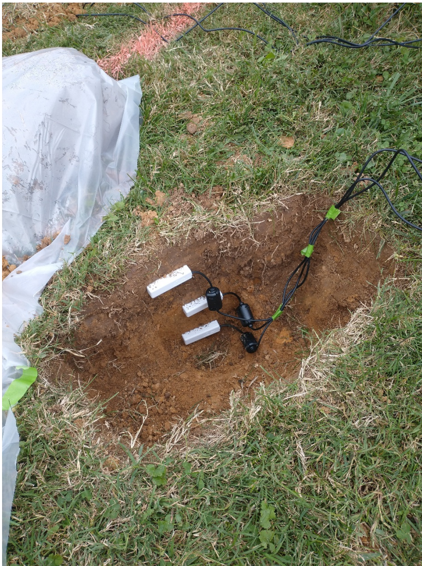
Figure 5 Vertically nested soil moisture sensors
