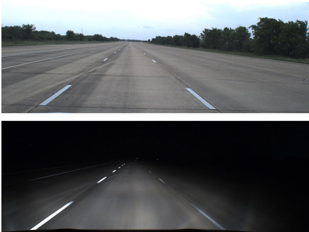
Figure 5: Images of 40 ft gap pavement markings on 35L (Set 2: 06W-6 on left and 02W-6 on right) during day (above) and night (below).
