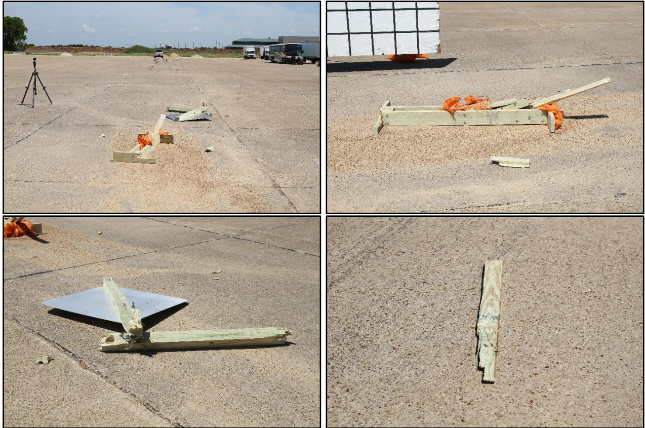
Figure 7.3. Modified TxDOT Single Skid-Mounted Sign Support after Test No. 469680-03-4.
