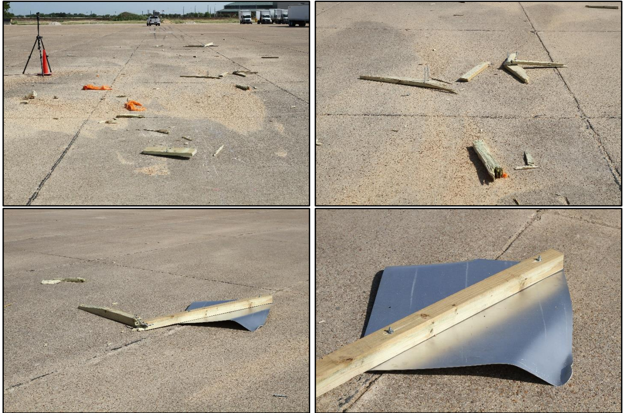
Figure 5.5. Modified TxDOT Single Skid-Mounted Sign Support after Test No. 469680-03-2A.
