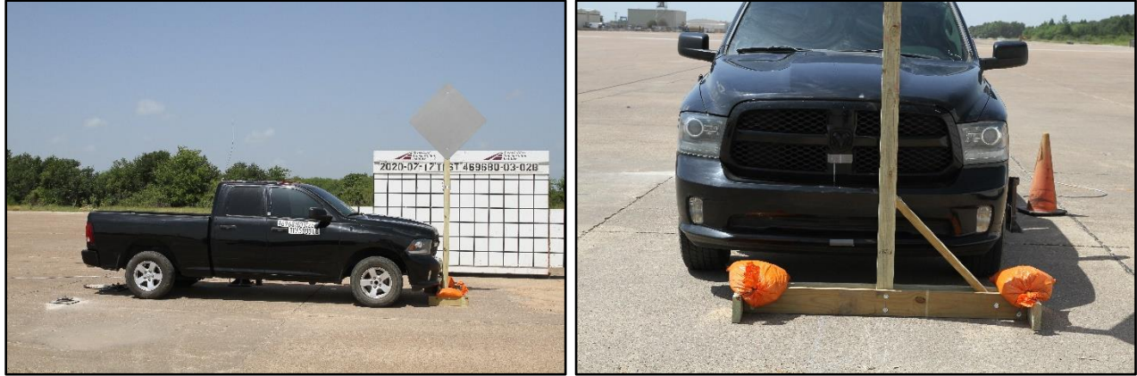
Figure 6.3. Sign Support/Test Vehicle Geometries for Test No. 469680-03-2B.
