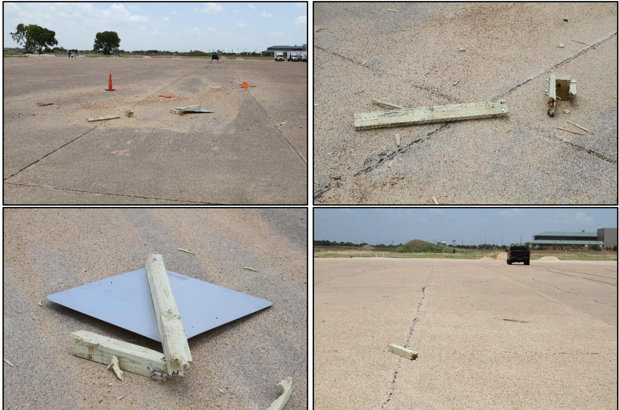
Figure 6.5. Modified TxDOT Single Skid-Mounted Sign Support after Test No. 469680-03-2B.
