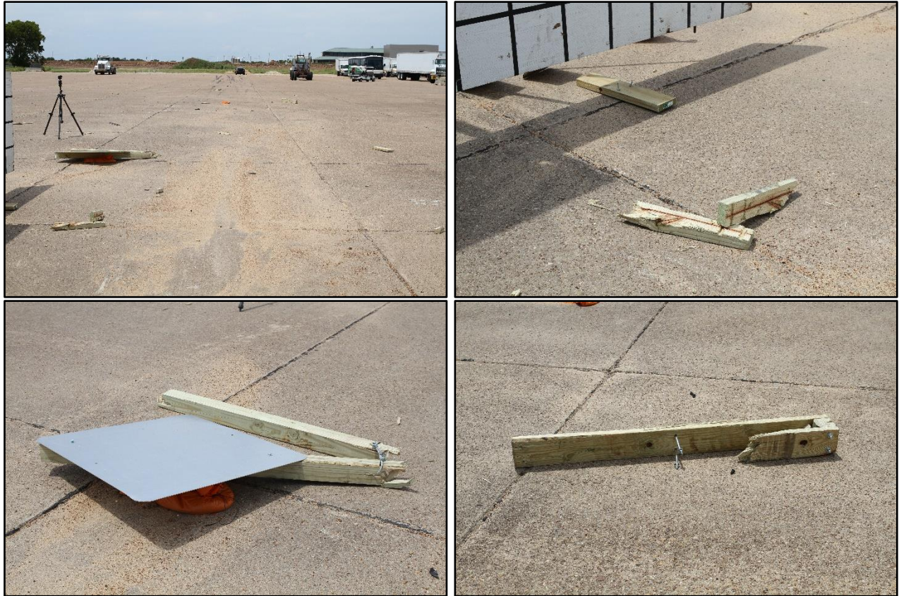
Figure 8.3. Modified TxDOT Single Skid-Mounted Sign Support after Test No. 469680-03-1.
