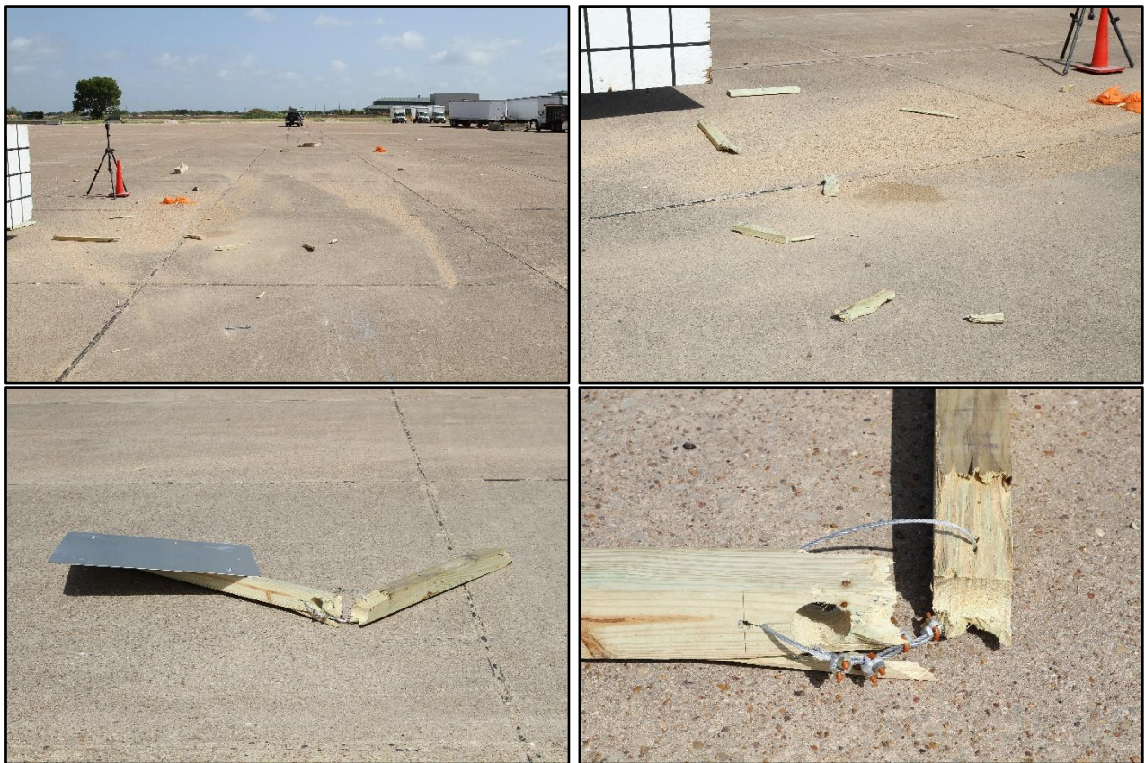
Figure 4.5. Modified TxDOT Single Skid-Mounted Sign Support after Test No. 469680-03-2.
