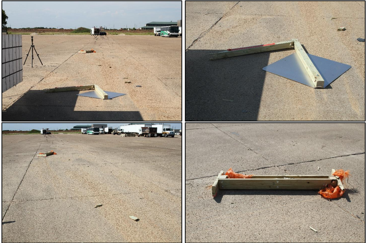
Figure 9.3. Modified TxDOT Single Skid-Mounted Sign Support after Test No. 469680-03-3.
