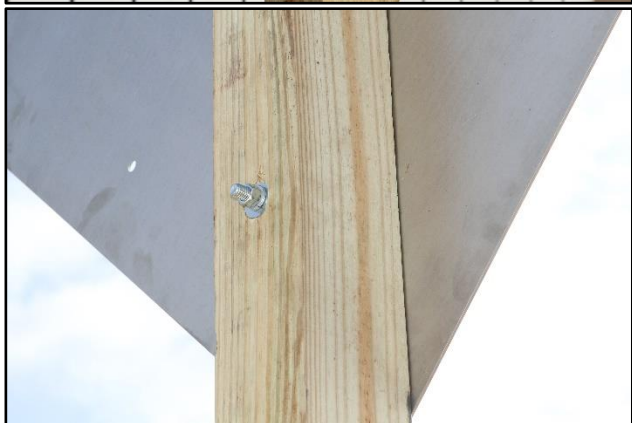
Figure 4.2. Modified TxDOT Single Skid-Mounted Sign Support (Original) prior to Crash Test No. 469680-03-2.
