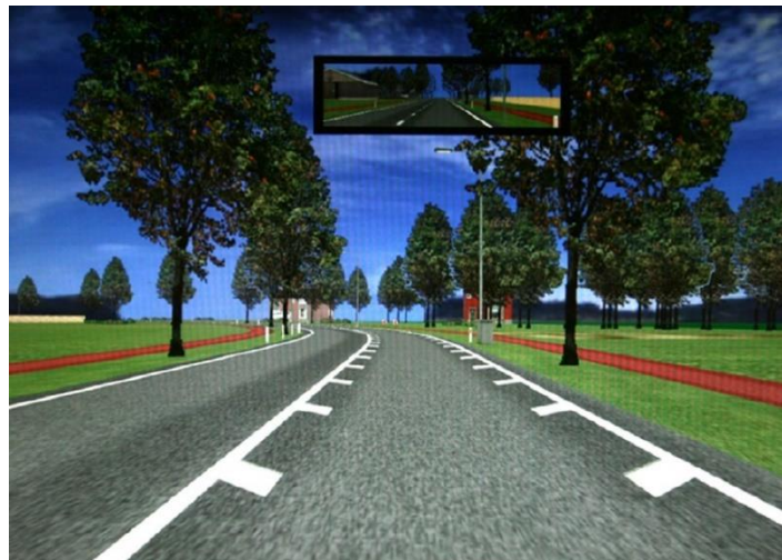
Figure 20. Herringbone-Pattern Optical Speed Bars (23).
