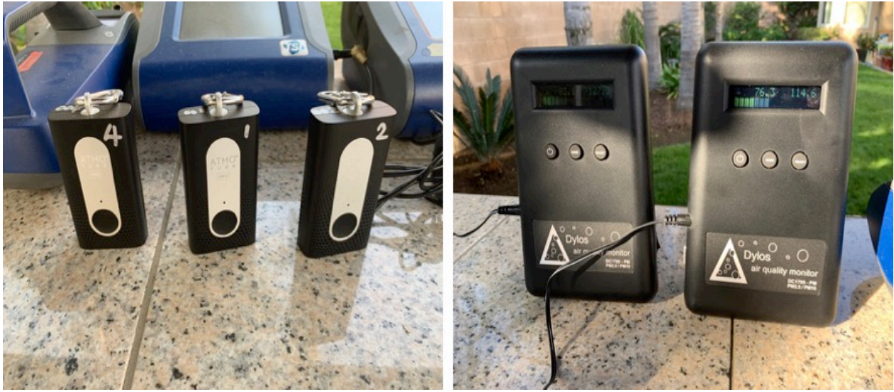
Figure 20. Low-cost Particulate Matter Air Sensors. (Left) AtmoTube Pro. (Right) Dylus DC1700
