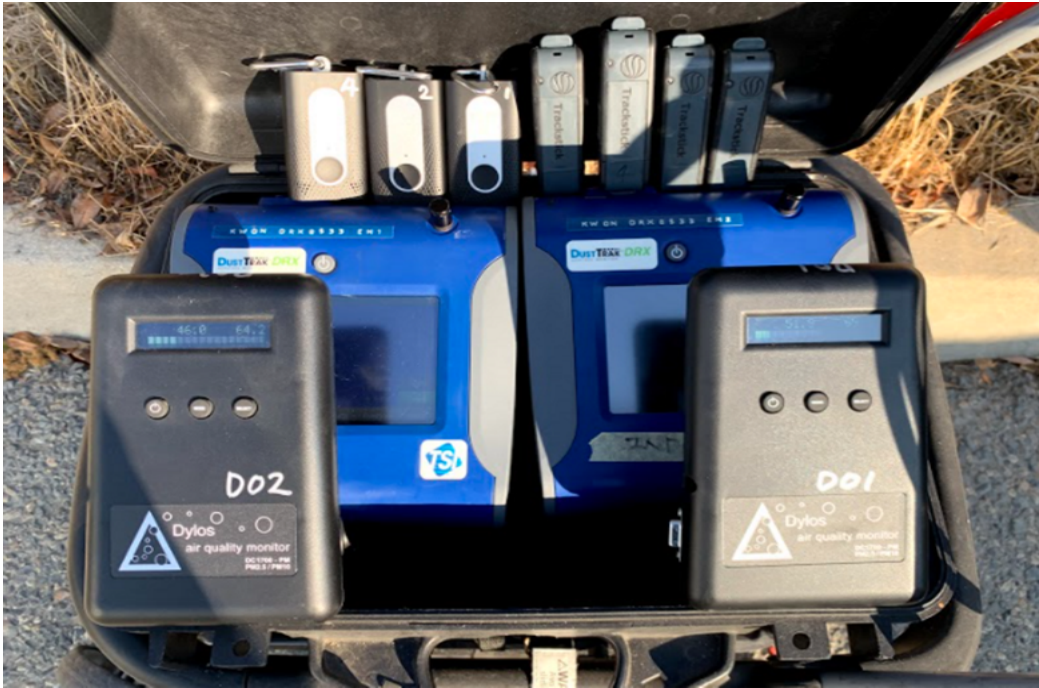
Figure 10. The Real-Time Portable Air Quality Monitoring Sensors: DRX Dusttrack 8533 Aerosol Monitors (TSI Inc., Shoreview, MN); Dylos DC1700 (Dylos Corp., Riverside, CA); Atmotube Pro (Atmotech Inc., San Francisco, CA); And Tracksticks.
