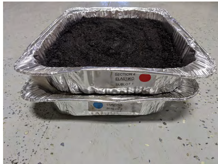
Figure 21: Pans used and Filled with Asphalt Mixture for Uniform Aging
