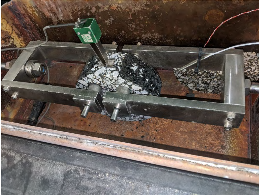
Figure 8: Disk-Shaped Compact Tension Testing Machine
