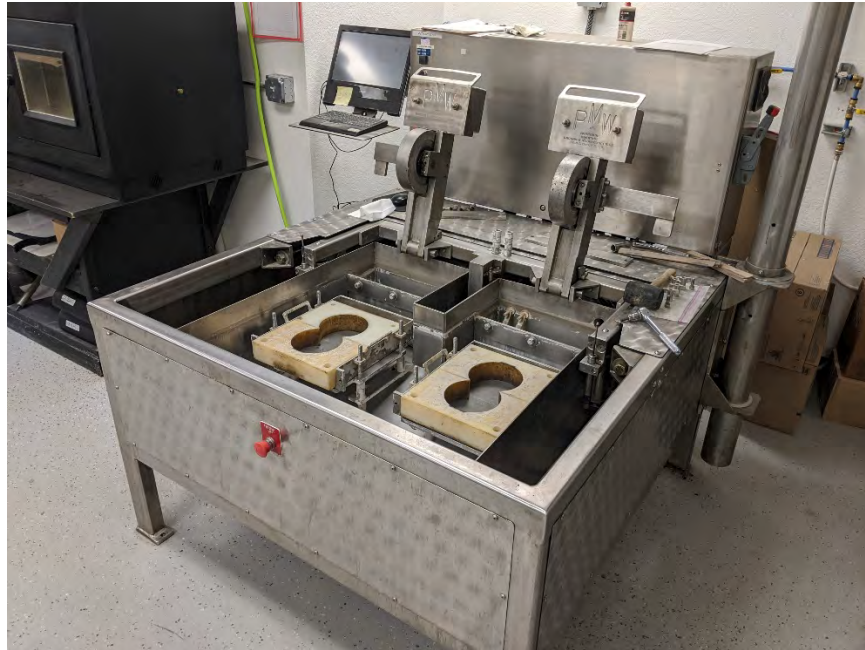
Figure 7: Hamburg Wheel Tracking Testing Machine
