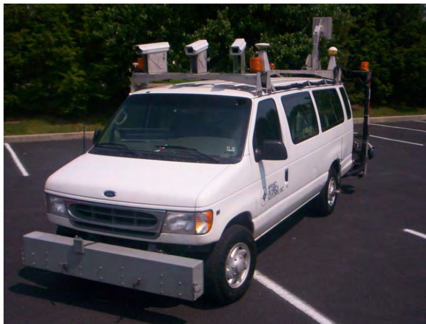
Figure 15: Digital Survey Vehicle Used to Measure Pavement Distresses
