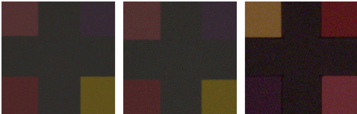
(a) Additive white Gaussian noise, \sigma = 0.0093 . (b) Intensity-dependent Gaussian noise, \sigma = 0.0499I + 0.00666 . (c) Real image noise example from SIDD.
