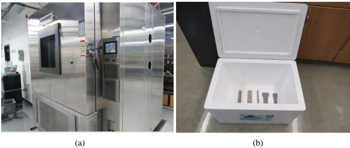
Figure 3.1 Conditioning of the specimens (a) temperature-humidity controlled chamber and (b) Styrofoam cooler
