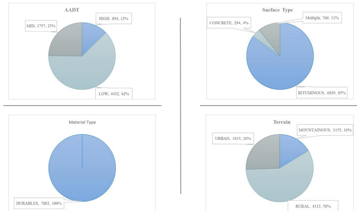
Figure 19. Road feature surveyed in Region 1 for AADT, Surface Type, Material Type and Terrain. In each inserted figure, the callout indicates feature, total mileage, and percentage.
